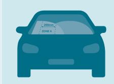
**Zone A:** it is a vertical area 290mm wide, centred on the steering wheel and contained within the swept area of the windscreen (this area is 350mm wide on vehicles over 3.5 tonnes).
